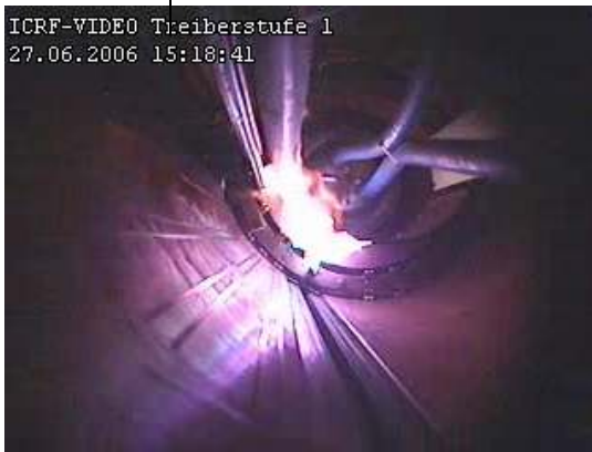
Arc in generator of ASDEX Upgrade
