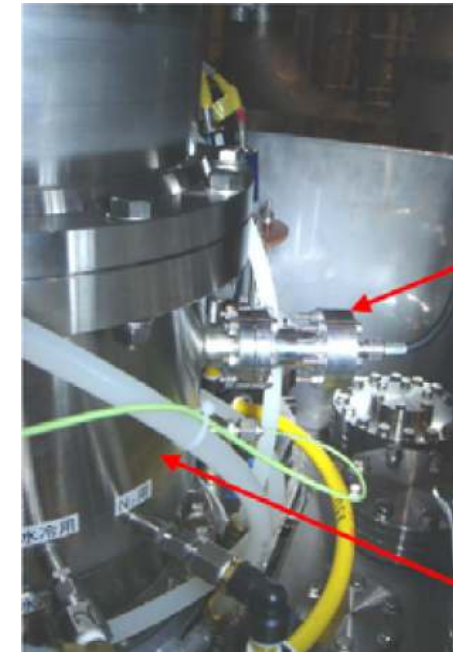
Optical detector for the vacuum feedthrough on LHD
