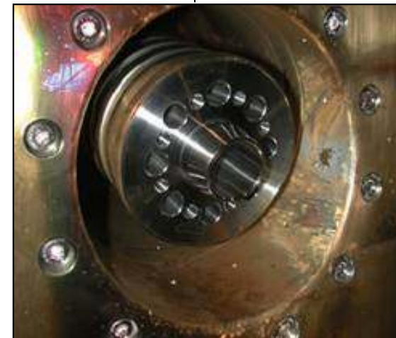
Antenna feeder – ASDEX Upgrade
